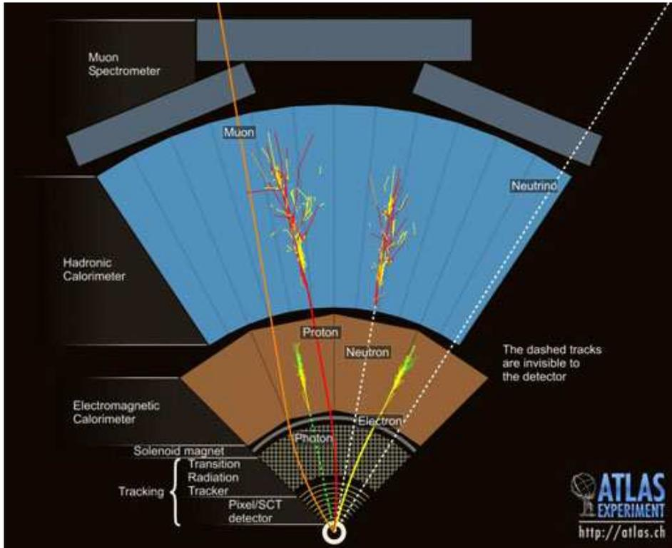
Figure 15: Particle reconstruction in the ATLAS detector. Particles leave signals in different parts of the detector and can be identified from this.
