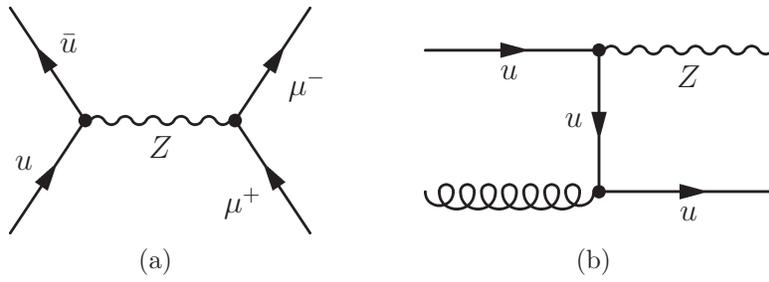
Figure 8: Examples to produce  $Z$ 's at a proton-proton collider. A quark and an antiquark makes a  $Z$  in figure 8a and a  $Z$  plus jet event is in figure 8b. The  $Z$  will decay before it reaches the detector.
