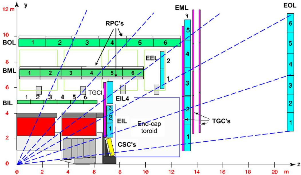
Figure 14: ATLAS Muon Spectrometer. The first letter of the MDT naming scheme refers to barrel and end-cap chambers while the second refers to inner, middle and outer layer.
