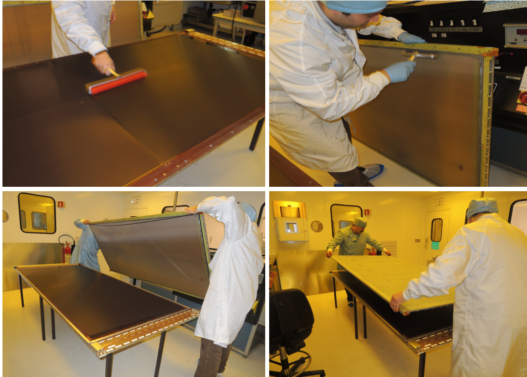
FIGURE 8.8: Top left and right: The active surface of the read-out panel and the floating mesh is cleaned with a static roller. Bottom left and right: The L2 chamber is closed by joining the two panels together.
