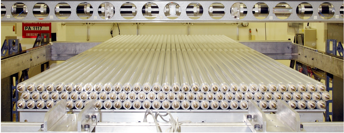
FIGURE 4.8: A MDT multi-layer under construction [8].
