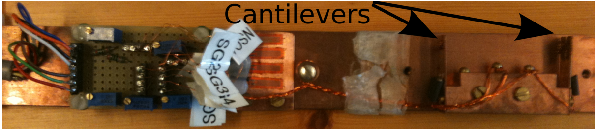
Figure 5.9: The setup with four cantilevers and dummy strain gauges as resistors. To the left one can see the four blue potentiometers, next to them are the four dummy strain gauges glued on an little copper plate. To the right the four cantilevers with strain gauges and - on some of them samples - are placed.
