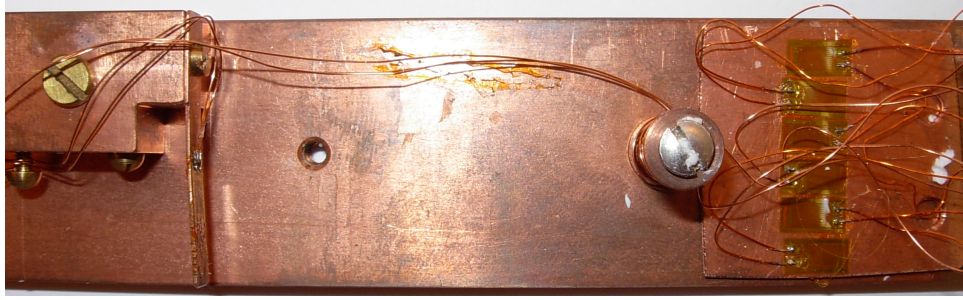
Figure 5.23: The final setup. To the left the cantilever with strain gauge, to the right the six dummy strain gauges needed in order to have two cantilevers with two Wheatstone circuits.
