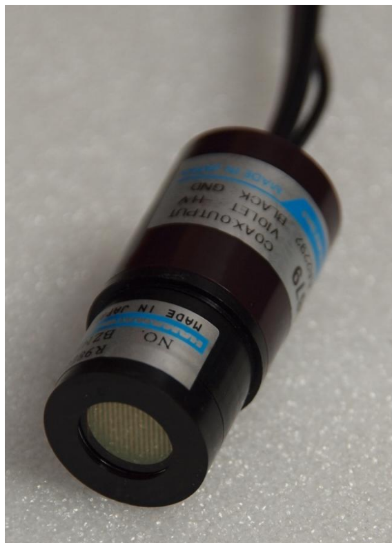
Figure 13.26. Hamamatsu R9880U-110 with voltage divider.
