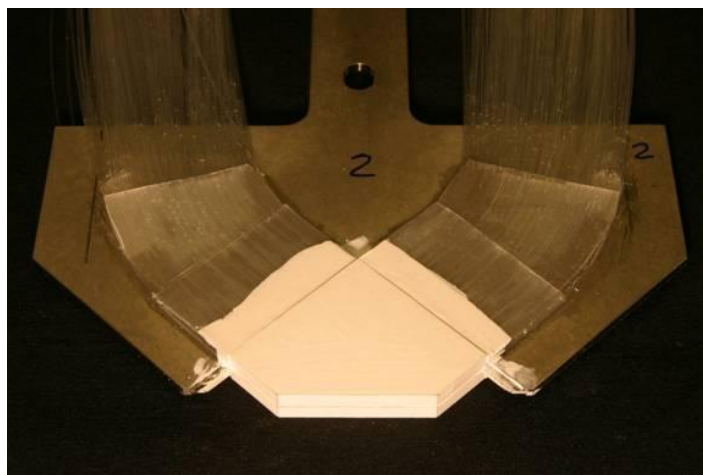
Figure 13.21. Titanium substrates with two main trigger scintillator tiles. These scintillator tiles each has two bundles of clear fibers connected to the two largest surfaces. The clear fibers for the bottom scintillator tiles are on the back of the titanium substrate. The figures is from [42](Detector production slide 17, H. Stenzel).
