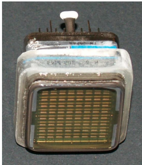
Figure 17.3. 3 rd generation shim: Epoxy glue.
