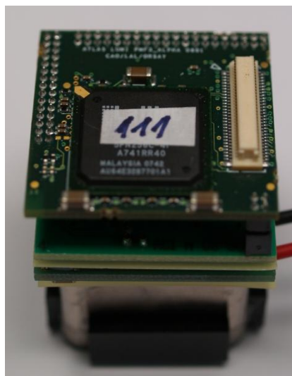
Figure 13.30. MAPMT with full PMF mounted: MAPMT + isolator + spacer + voltage divider + spacer + isolator + passive board + active board.
