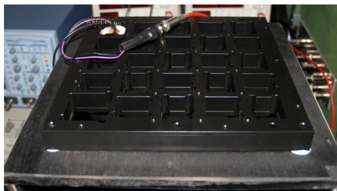
Figure 16.18. The mu-metal grid frame made in POM with the Teflon piece holding the PMT.
