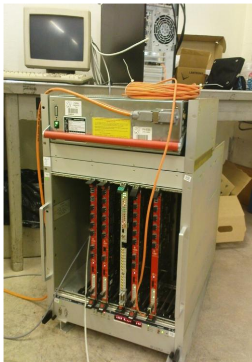
Figure 13.35. The WME create with the DAQ system. The figure is from [42](Back End and DAQ, G. Blanchot and K. Korcyl slide 5).
