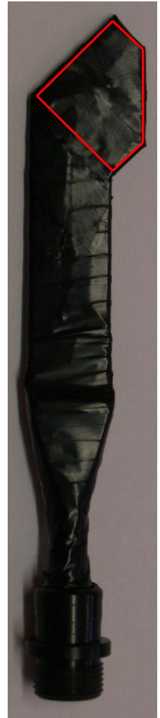
Figure 14.10. LEFT: The 2005 prototype with 4 layers of fibers. The overlap (the detecting area) of the fiber layers are pointed out in red. RIGHT: Trigger scintillator tile with light guide. The shape of the scintillator tile is pointed out in red.
