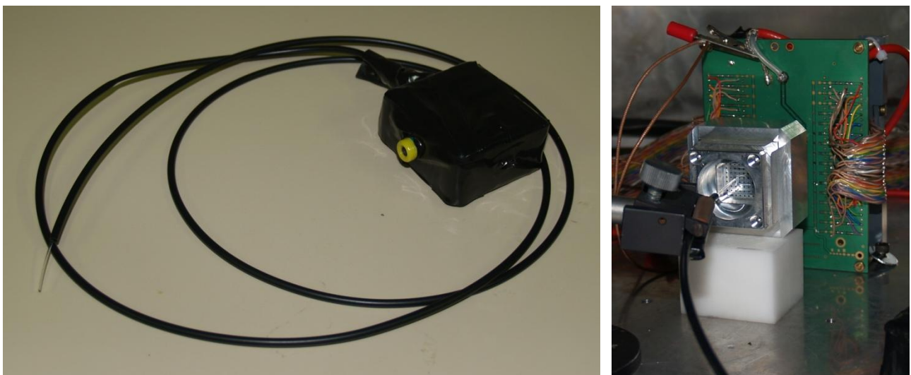
Figure 14.6. LEFT: LED mounted in a metal box and a light guide to get the light out of the box. RIGHT: Aluminum piece mounted on the MAPMT and the light guide place in front of it.
