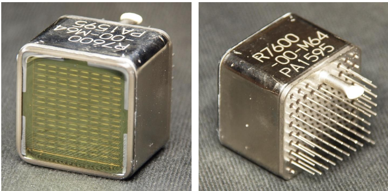
Figure 13.18. LEFT: The MAPMT from the front. The windows of each channel are shown. RIGHT: The MAPMT from the back. The vacuum pin (white) and the pins are shown. The center 64 pins are for each MAPMT channel. The outer pins are the voltage for each dynode.
