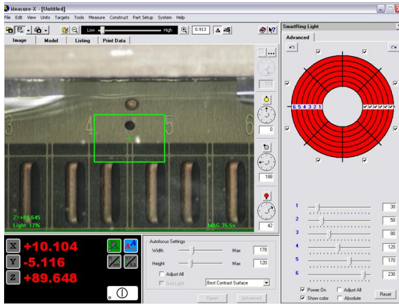
Figure 17.7. Screenshot from the digital microscope used for finding the position point on the top plate and the moved to the position where the precision point of the MAPMT channel-grid should be.
