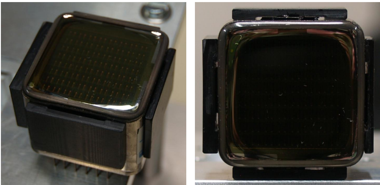
Figure 17.8. LEFT: MAPMT with shims as “proof of method”. RIGHT: MAPMT with shims as “proof of method”. It is shown that the glue fill out the space foreseen for it and the distance is defined by the shim (not the shim + glue).
