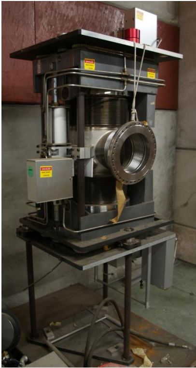
Figure 13.36. LEFT: A Roman Pot station from the UA4 (SPS) experiment. RIGHT: The Roman Pots from the UA4 (SPS) experiment.
