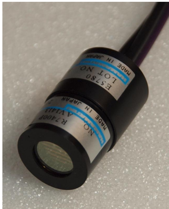
Figure 13.24. Hamamatsu R7400P PMT with voltage divider.
