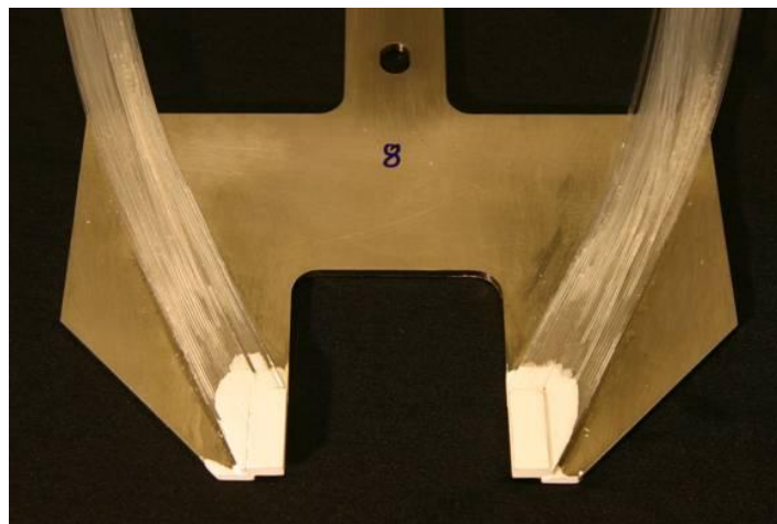
Figure 13.23. Titanium substrates with two overlap trigger scintillator tiles. These scintillator tiles have a bundle of clear fibers connected. The figure is from [42](Detector production Slide 17, H. Stenzel).
