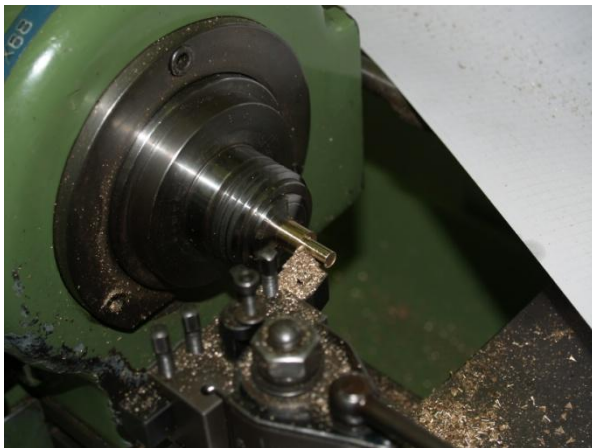
Figure 15.3. LEFT: One of the brass spacer being made on a lathe. RIGHT: Holes being drilled in the aluminum plates.
