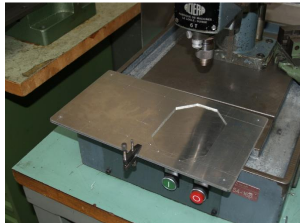
Figure 15.3. LEFT: One of the brass spacer being made on a lathe. RIGHT: Holes being drilled in the aluminum plates.
