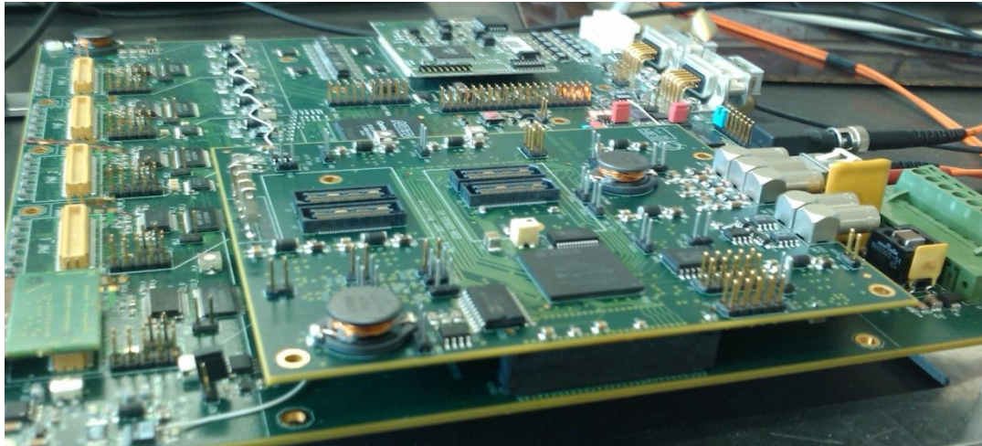
Figure 13.34. The ALFA trigger mezzanine mounted on the ALFA motherboard. The figure is from [60](slide 6).
