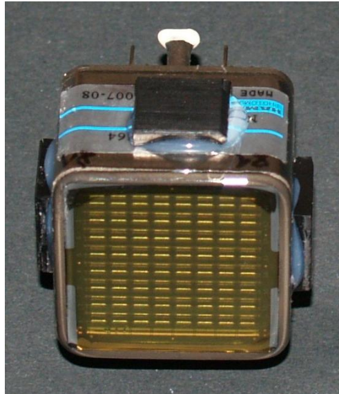
Figure 17.2. 2 nd generation shim: Flat piece of POM glued to the MAPMT.
