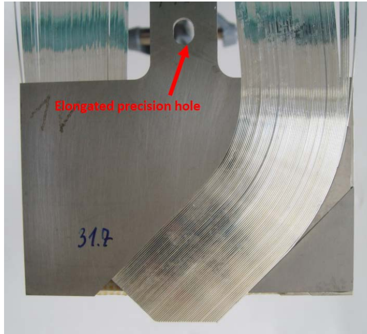
Figure 6.2: Picture of a titanium plate with the fibers for the V(U)-plane glued to the front(back).
