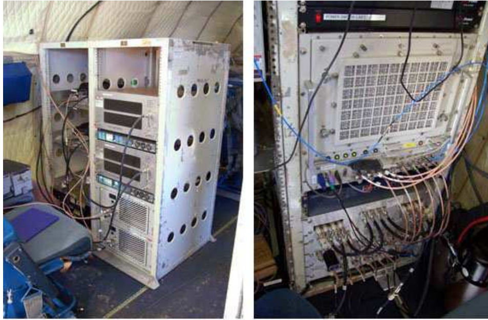
Figure 2.1: Radar power amplifiers (left) and electronics chassis (right) installed inside the P-3 aircraft. Photos from Jezek et al. (2007).
