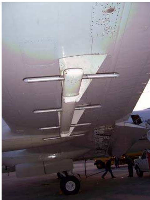
Figure 2.2: Four 150 MHz dipole antennae mounted under the right wing of a P-3 aircraft. Photo from Jezek et al. (2007).
