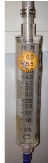
Figure 6: Ping pong flow meter
