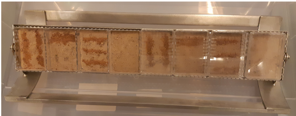
Figure 5: Image showing the arrangement of perchlorate rich soil at initiation of experiment, testing the setup. From the left, the first four boxes are without holes, box five to eight are with holes and lids on.
