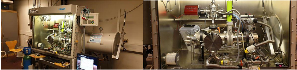
Figure 9: The Jens Martin Mars Chamber glovebox. To the left the figure includes the control panel and the airlock. To the right is a close up of the actual Mars chamber.
