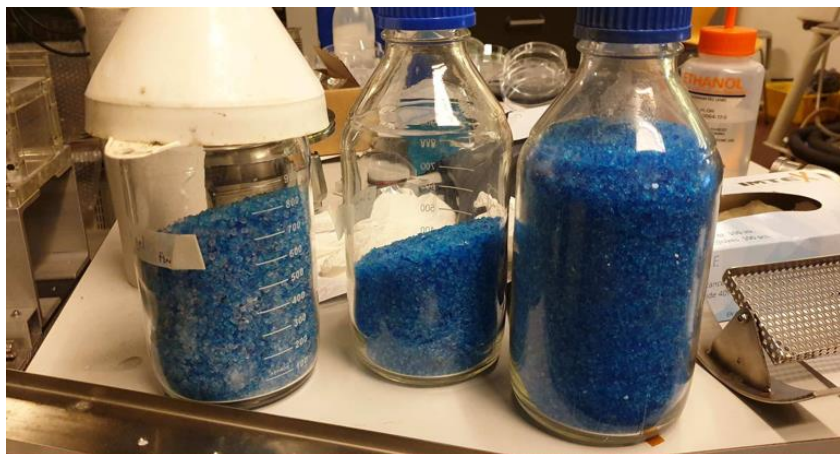
Figure 11: The silica gel used to lower humidity.
