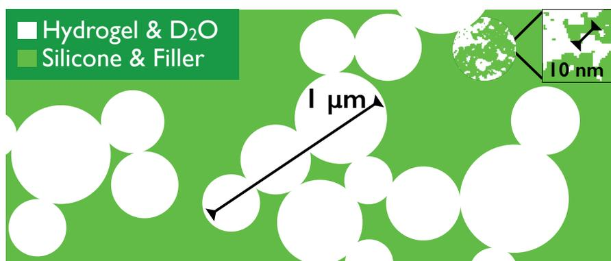
While the previous SANS experiments studied the IPN structure on a nanometer length scale, SESANS measurements probe inhomogeneities in the micrometer range. The results revealed that the material is divided in spherical regions of hydrogel-rich material in otherwise hydrogel-poor material.
