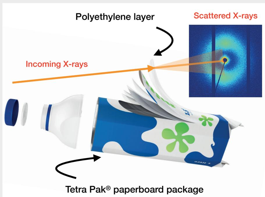
Polyethylene layers act as a barrier and adhesive for Tetra Pak® paperboard packages. X-ray scattering measurements on one of the polymer films show that crystals in some films have a preferential orientation originating from the process used to produce them.
