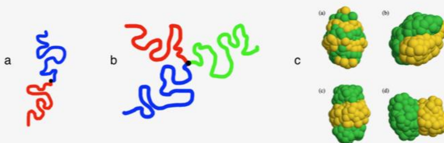
Figure: (a) An AB diblock copolymer (b) An ABC miktoarm terpolymer. (c) Single chain structures formed by a AB_n diblocks (a chain of AB 's) in poor solvent for both blocks A and B.
