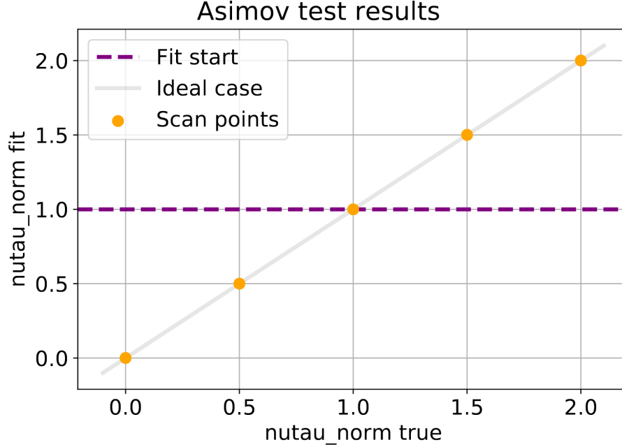
Figure 72: Result of the injection-recovery test on Asimov datasets. For each of the scan points shown in yellow, a fit was performed where the pseudo-data is generated with a different true tau normalization value. The purple dash line represents where the initial tau normalization value of the MC template, prior to the fit.
