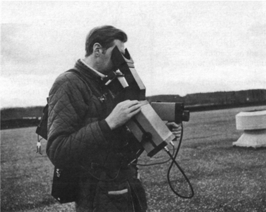
Infrared roof moisture monitoring equipment.
