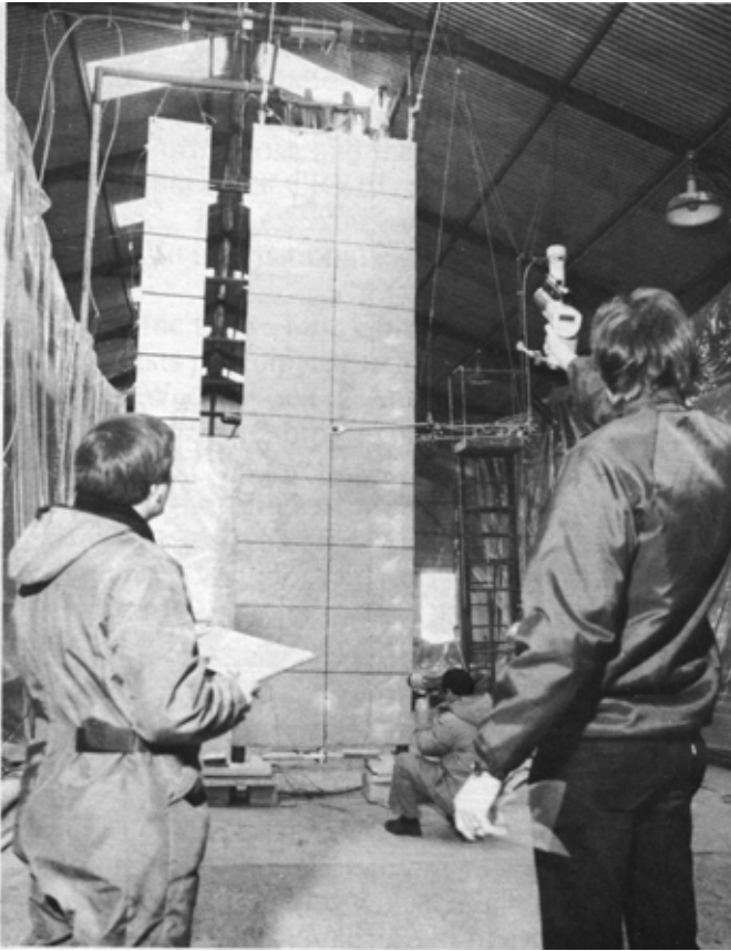
Testing cryogenic panel (for the Space Shuttle) at CRREL.
