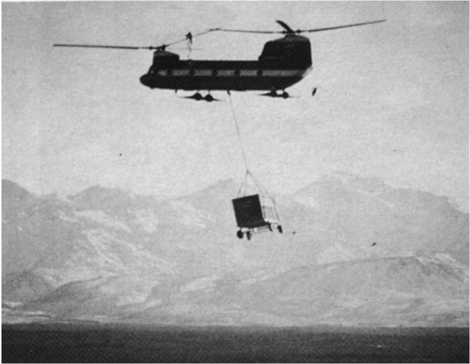
Air-transportable shelter for Arctic use
