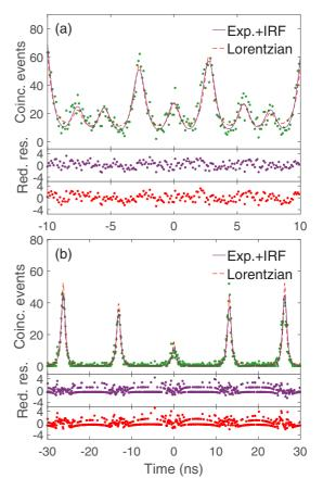
FIG. 10. Two-photon coincidence data at 4.2 K for 2.7-ns (a) and 13-ns (b) path delay. The peaks are fitted with either double-sided exponentials convoluted with the measured instruments response (solid purple) or a Lorentzian (dashed red) by optimizing the Poisson MLE. The corresponding reduced residues for each fit are shown below the figures.
