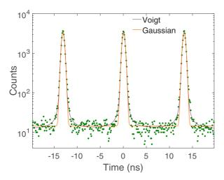
FIG. 9. The measured instrument response function (IRF) of the Hanbury Brown and Twiss setup fitted with both a Voigt (purple) and a Gaussian (orange) function using the Poisson MLE described in the text. The Voigt function with its broader tail provides a superior fit to the line shape of the IRF evidenced by the smaller  $\chi^2_{MLE}=2.3$  vs 5.7 for the Gaussian fit.
