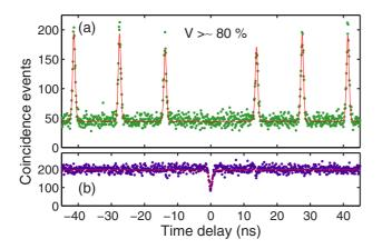
FIG. 7. HOM correlation histograms of device C in the case of strict resonant excitation with 100-ps-long pulses at  $0.8P_{\rm sat}$  (a) and with continuous-wave excitation at  $0.5P_{\rm sat}$  (b). The operation temperature of the experiment is 1.58 K. The fit of the experimental data to theory is shown by the red line.
