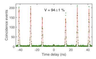
FIG. 6. Coincidences histogram of the HOM interference data recorded on device C under quasiresonant excitation for a successive time separation of emitted photons of  $\sim$ 13 ns, measured at 1.7 K and at  $P_{\rm sat}$ . The data points present the raw data without any background correction. The fit of the experimental data to theory is shown by the red line.
