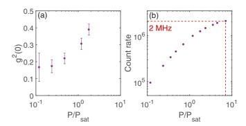
FIG. 5. Efficiency of a single-photon source with no electrical gates (device B). (a) Autocorrelation function at zero time delay  $g^2(0)$  vs excitation power measured in units of the saturation power  $P_{\text{sat}}$ . (b) Raw count rate on an avalanche photodiode as a function of excitation power. A count rate of up to 2 MHz is observed, where about half of it stems from the QD.
