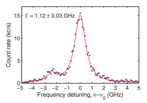
FIG. 8. Resonance fluorescence of a quantum dot vs laser frequency detuning. The data are recorded at a power of  $0.2P_{sat}$  at 1.58 K. The resonance frequency  $\nu=325.457\,\text{THz}$  corresponds to a wavelength of 921.14 nm. The solid line is a Lorentzian fit to the data with linewidth  $\Gamma=1.12\pm0.03\,\text{GHz}$ . The weak peak on the lower-energy side stems from another QD dipole weakly coupled to the waveguide.
