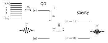
FIG. 1. Schematic of the cavity QED system including the phonon interaction. The QD-cavity coupling strength is g and the QD-phonon interaction matrix elements are  $M_k$ . The rates  $\Gamma$  and  $\kappa$  yield decay of the QD and cavity, respectively. Pure dephasing of the QD is included through  $\gamma$  and  $\Delta$  is the QD-cavity detuning.
