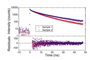
FIG. 8. (Color online) Decay curves for quantum dot samples with different SiO<sub>2</sub> layer thicknesses z=73 nm and z=166 nm, respectively, for samples 1 and 2 measured at an emission energy of 2.08 eV. The decay curves are fitted with a lognormal distribution of decay rates. Residuals are shown in the bottom panel.
