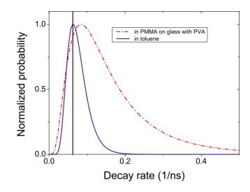
FIG. 7. (Color online) Lognormal distribution of decay rates of quantum dots in a PMMA layer on glass with a PVA cover layer and for quantum dots in toluene resulting from fits in Fig. 6. The black line shows the delta function distribution for single exponential fit.
