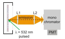
FIG. 4. (Color online) A schematic picture of the experimental setup. Light from the laser excites the quantum dots in a layered sample inside a nitrogen purged chamber. The emitted light is collimated by a lens L1 with f=12 cm, focused by lens L2 with f=10 cm on the entrance slit of a monochromator, and detected by the photomultiplier tube.
