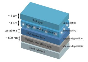
FIG. 1. (Color online) Schematic cross section of the sample used in the measurements. The different layers of the sample are shown together with corresponding thickness and fabrication technique.
