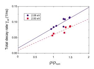
FIG. 11. (Color online) The decay rate versus the normalized isotropic LDOS for two different emission energies. Data are fitted with a linear function as expected from Fermi's golden rule.
