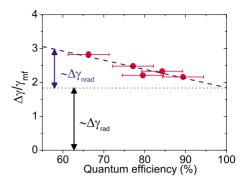
FIG. 14. (Color online) Measurements of relative width for a homogeneous system (LDOS=1) plotted versus the extracted quantum efficiency [see Fig. 12(b)] together with a linear fit.
