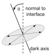
FIG. 10. The angle  $\theta$  is the angle between the dark axis of the CdSe quantum dot and the normal to the interface.
