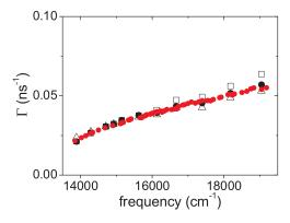
FIG. 3 (color). Radiative decay rate from tight-binding calculations (red dots) for CdTe [same experimental data as in Fig. 2(a) are plotted].
