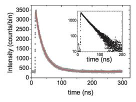
FIG. 1 (color). Luminescence decay curve of exciton emission from CdSe nanocrystals at 620 nm  $\pm$  5 nm (filled circles). Single-exponential fit (red curve), with background as adjustable parameter, yields a rate of  $0.037 \pm 0.003$  ns<sup>-1</sup> and a  $\chi_r^2$  value of 1.4. A stretched-exponential model yields a rate of 0.036 ns<sup>-1</sup> and a  $\beta$  value of 0.99. Inset: the background corrected decay curve in a semilogarithmic plot.
