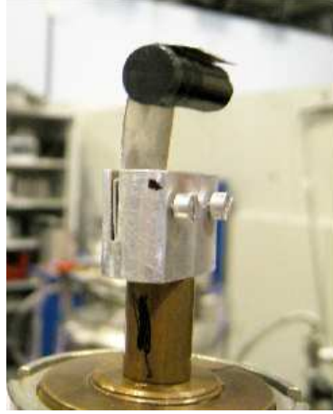
Figure 5.4: Picture of our sample. The black dot indicates the (1\ 0\ 0) axis.
