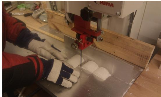
Figure 3.1: Here the 5 cm samples are getting cut and prepared for further measurements.
