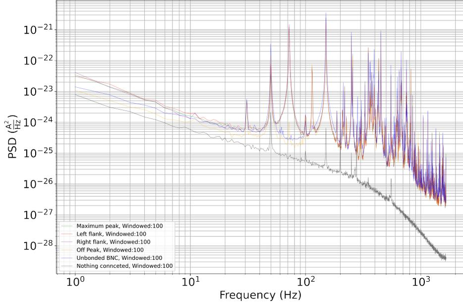
Figure 14: Higher frequency power spectral density using 100 windows averaged together, resulting in 1 s time traces. Data acquired from device QBB16\_3\_5.
