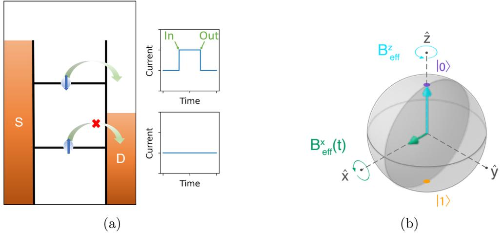
Figure 1: Loss-DiVincenzo spin qubit (a) Diagram of the electrochemical potential, showing that the higher energy state is allowed to tunnel to the drain, while the lower is not. (b) Bloch sphere showing a time varying magnetic field  $B_{eff}^x(t)$  rotates the state around the x axis, while a static magnetic field  $B_{eff}^z$  rotates it around the z axis [3]
