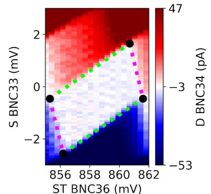
Figure 6: Close-up of the SiGe Coulomb diamond used to extract data. The lime green lines represent the slope  $\beta$  and the magenta lines represent the slope  $\gamma$ . Data acquired from device D21 10B (T2) 24\_3.3.
