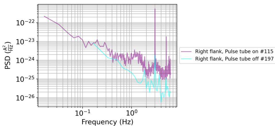
Figure 17: Noise spectra, as obtained in 7.3, but with pulse tube cooler temporarily turned off for #197
