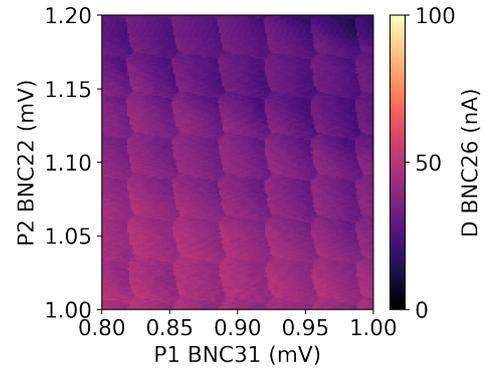
Figure 15: Plunger sweeps of the double dot in the SiMOS device. Data acquired from device QBB16\_3\_5.
