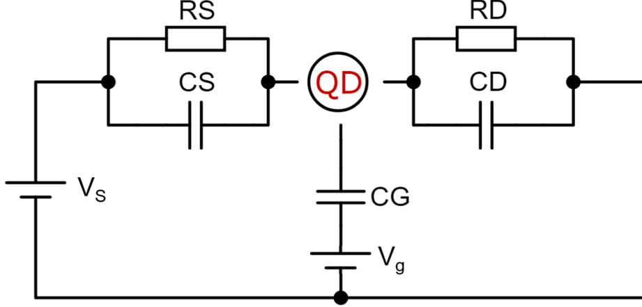
Figure 2: Circuit Diagram of a quantum dot, the tunnel junctions consist of a resistor and capacitor connected in parallel, and the gate is defined by a single capacitor.
