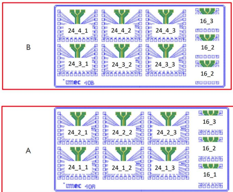
Figure 16: Locations of several SiGe Devices and their bonding pads on chip A and chip B. ID of SiGe wafer: AL902605 Die 2. Image provided by IMEC.
