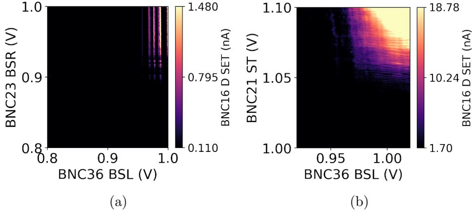
Figure 10: Measurements of a diagonal design device where a positive voltage is applied to all SET gates. (a) Barrier/barrier sweep showing a strong coupling to BSL. (b) Sweep of the barrier gate BSL and the ST gate. Data for Fig. (a) and (b) was acquired from device D20 10B (T3) 16\_3.
