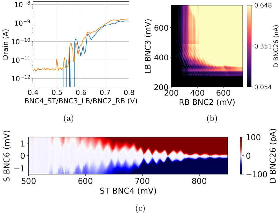
Figure 12: (a) Activation of the SiMOS device in log scale. Bias = 0.3 mV. (b) Barrier sweeps of SiMOS showing clear Coulomb blockade at the region where the voltage on the barriers are approximately 400 mV. (c) Coulomb diamonds of a SiMOS device. Data acquired from device QBB16\_3.5.
