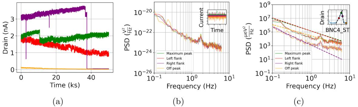
Figure 8: (a) Time traces from different positions of a Coulomb peak, due to large charge jump the position of each trace is shifted (b) 100s time traces converted to a power spectral density in units of  $\frac{V^2}{Hz}$ . Inset: time traces (c) Power spectral density in  $\frac{\mu eV^2}{Hz}$  with  $\frac{A}{f^\beta}$  fit. Values of  $\beta$  in fits on graph (c) descending order of its legend: 1.81, 1.92, 3.15, 1.63. Data acquired from device D21 10B (T2) 24.3.3.
