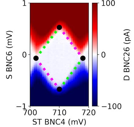
Figure 11: Close-up of the SiMOS Coulomb diamond used to extract data. The lime green line represent the slope  $\beta$  and the magenta line represent the slope  $\gamma$ . Data acquired from device QBB16\_3.5.
