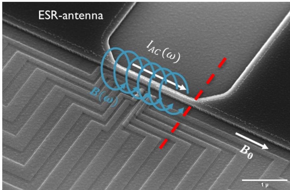
Figure 18: SiMOS SEM image, illustrating how an AC current through the ESR antenna creates an AC magnetic field  $B(\omega)$  at the qubit location, perpendicular to the static applied field  $B_0$ . Image provided by IMEC.
