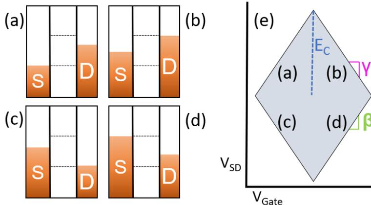
Figure 3: Source/Drain alignment at each slope in a Coulomb diamond. For actual data obtained in this regime, see Fig. 6
