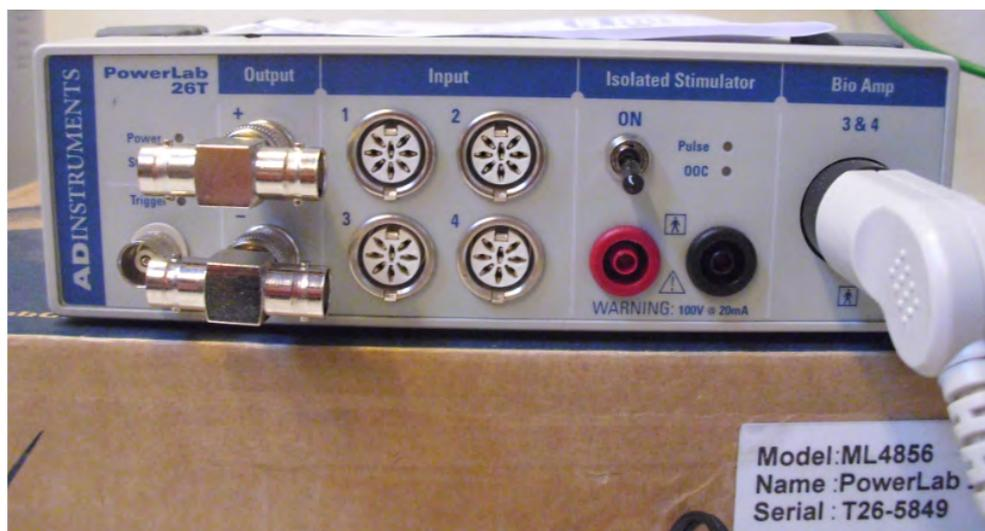
Figure 2.6: PowerLab 26T. In the left the output connection, used for the generation of the stimulation signal, while in the right the Bio-amplifier is connected to the recording channels.
