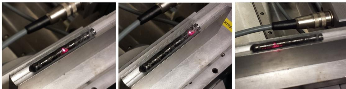
Figure 11: Pictures of  $x = 0.04$ . Three different measurements on the same crystal are shown. The red spot marked the striking point of the beam.
