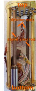
**Figure 4:** Photo of the inside of a puck with the current stabilizing rods and no sample. Cables are from an old experiment and will be changed when the new sample system arrives.
