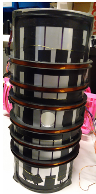
Figure A.1.: picture of the coil system around aluminum layer of shield
