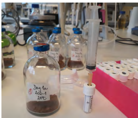
Figure 24: Residual gas extraction
