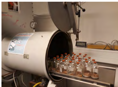
Figure 23: Samples inserting the GB through the airlock
