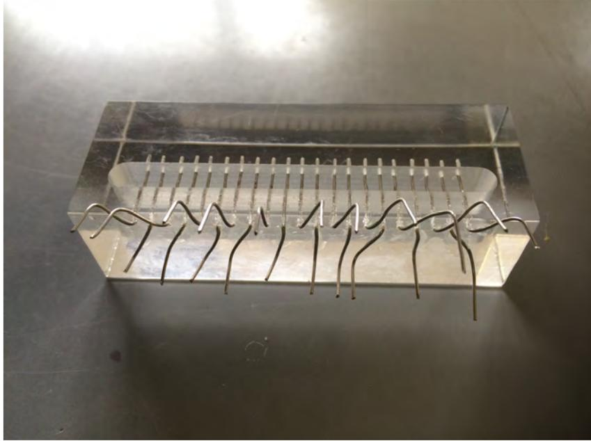
Figure 21: Picture of the recording chamber used in the collision experiments. The chamber is carved from a 2 by 7 cm block of acrylic glass. The groove is 6 cm in length, 0.5 cm wide and 1 cm deep. 21 electrode wires are inserted into the chamber in equidistant spacing of about 0.25 cm. The electrodes are made of resistance wire with a resistance of  $5.40\Omega/m$  at  $20^\circ C$ .
