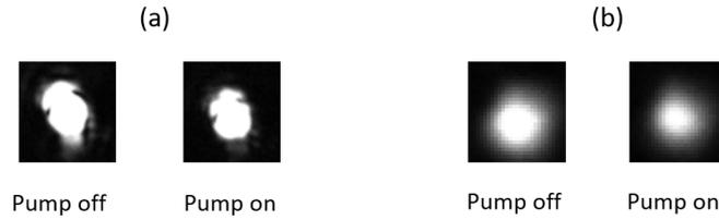
Figure 5.4: Camera mode of the 930 nm light with the pump on and off for (a) a situation with higher order modes present and (b) a situation without higher order modes present
