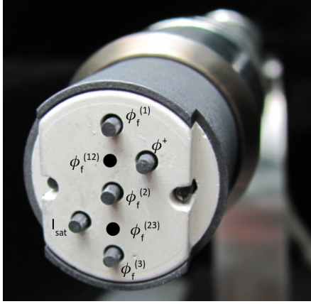
(a) From [12], image of a probe used in the EAST experiments. The different tips are marked with the corresponding name of the obtained signal. The values \phi_f^{(12)} and \phi_f^{(23)} are not measured but obtained from averaging the signals from the corresponding upper and lower tips.
