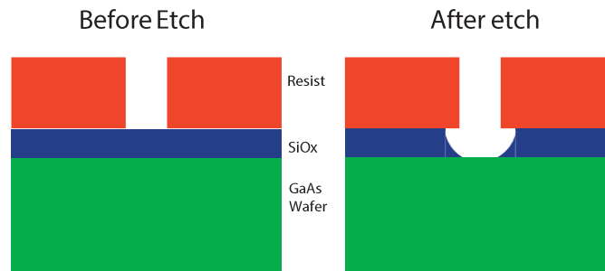
Figure 13: The illustration shows a before and after isotropic HF etch schematic. The before etch illustration shows the step after development of the resist and before etch. After etch the SiOx has been removed in a pattern characteristic for isotropic etching (etching in all directions).
