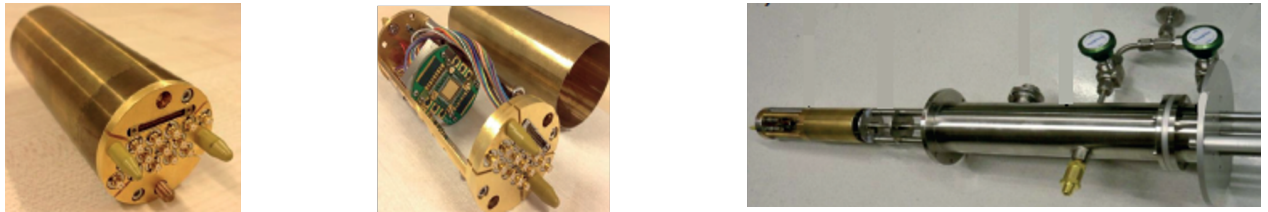
Figure 4.19: Left , a picture of the puck. Middle , a picture of the puck without the shield. The daughterboard containing the sample is mounted onto the motherboard, which has electrical connectors to both the bottom and the top of the puck, ensuring electrical connection to both the wiring inside the cryostat and the loading stick. Right , a picture of the loading stick with the puck mounted onto it. The loading stick is grounded to minimize the risk of blowing up a device, while attached to the puck.
