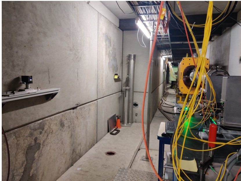
Figure 18: A photograph of the H8 extraction line. Seen on the left is the internal wall where the aligning laser originates from the light source placed at the yellow sticker in the photograph. The laser then hits the pentaprism seen to the left, which deflects it 90 degrees towards the crystal on the goniometer to the right.
