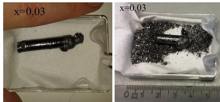
Figure 6.5: An example of a crystal sample as-grown (left) and after a few days left in air (right) kept in the same open container in air. Some white powder is visible after a few days, clearly indicating the presence of \text{La}(\text{OH})_3 .
