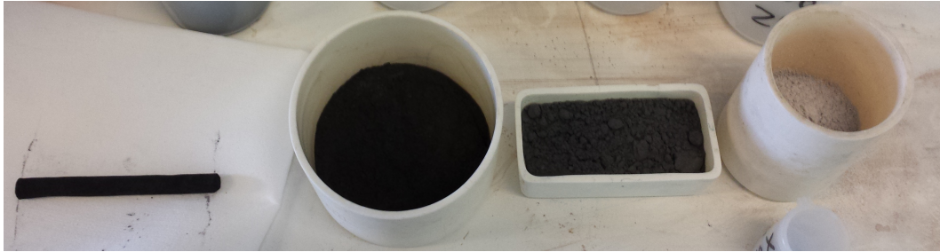
Figure 6.1: To the left, a pressed rod as it looks once removed from the silicone tube before sintering. The three powders to the right show the progression from right to left from initial mixing to after the second calcination.
