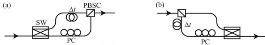
**Figure 2.9** (a) Time-Bin  $\rightarrow$  Polarization; (b) Polarization  $\rightarrow$  Time-Bin. The Polarization Controller (PC) rotates the polarization to match  $|H\rangle$  and  $|V\rangle$  states. The Switch (SW) flips the 2 paths periodically. An extra piece of wire delays the  $|E\rangle$  photon to match with the  $|L\rangle$  photon. Note that the circuit succeeds 50% of the time, just when the  $|E\rangle$  photon takes the long path.
