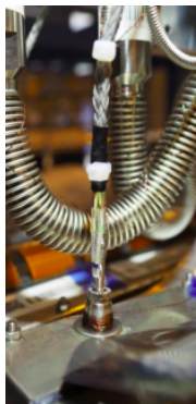
Figure 7.10: PT100 glued onto the dry gas outlet
