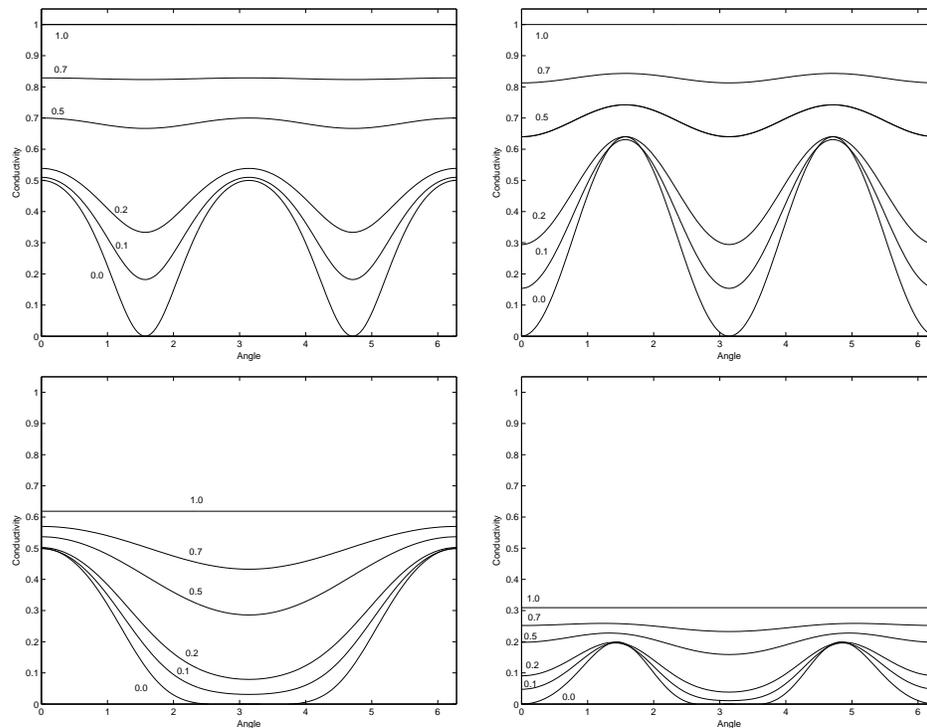
Figure 7.11: Graphs showing how the conductivities depend on the polarization of the leads. The numbers on the graphs show the polarization. The top left is the parallel coherent conductivity, the bottom left is the parallel correlated conductivity, the top right is the anti-parallel coherent conductivity and the bottom right is the anti-parallel correlated conductivity.
