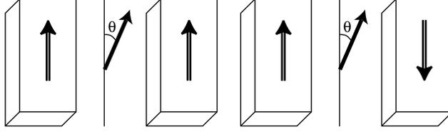
Figure 7.1: The geometry of the parallel and anti-parallel configuration of the contacts and the quantum dot magnetization with an angle  $\theta$  to the direction of the parallel magnetization.
