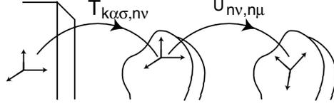
Figure 2.2: The coupling visualized. Read from left to right an electron tunnel into the dot (amplitude  $T$ ) and changes basis (amplitude  $U$ ). If the figure is read from right to left the opposite happens.
