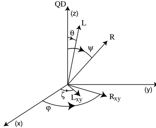
Figure 2.3: The four angles of rotation are shown. QD, R and L names the directions of the quantum dot, right lead and left lead magnetizations respectively.
