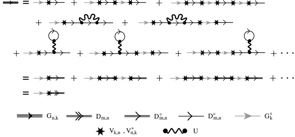
Figure 4.1: Decomposition of the current Green's function into the free lead and full dot Green's functions. The current Green's function is expanded in the tunneling and dot-interactions. As a model for the dot-interactions is used the Coulomb model discussed in chapter 6. The Green's functions used in the diagram are defined in the text except for the interacting dot-Green's function ( $D^U$ ) which is only used as an intermediate function.
