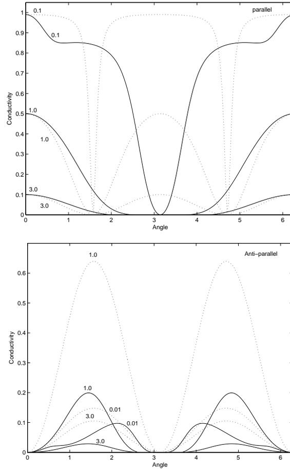
Figure 7.6: The level spacing dependence of the conductivity. The full lines are the correlated conductivities and the dotted lines are the coherent conductivities. The top figure is in the parallel configuration and the bottom one is in the anti-parallel configuration. The numbers on the curves are the level spacing. The  $y$ -axis is in units of  $\frac{e^2}{h}$ .
