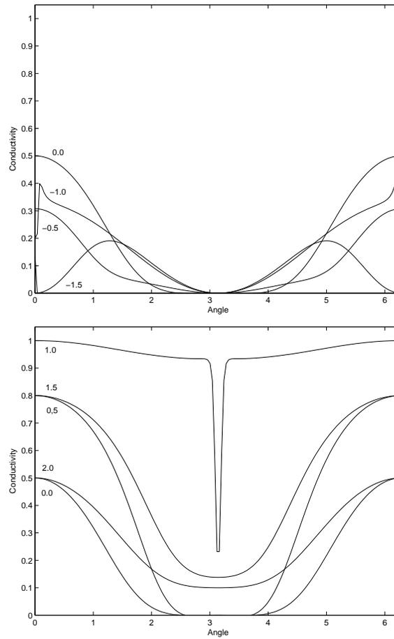
Figure 7.8: The gate dependence of the parallel correlated conductivity. The top figure shows the gates from  $-1.5$  to  $0.0$  while the bottom figure shows the gates from  $0.0$  to  $2.0$ . The numbers on the graphs is the gate energy. The  $y$ -axis is in units of  $\frac{e^2}{h}$
