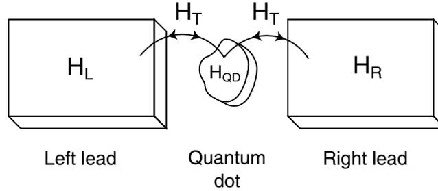
Figure 2.1: The figure illustrated the Hamiltonians of the system. The three regions (left and right contact and the quantum dot) have each their own Hamiltonian which only contains information about the respective region. Furthermore the coupling between the regions are described by a separate Hamiltonian.
