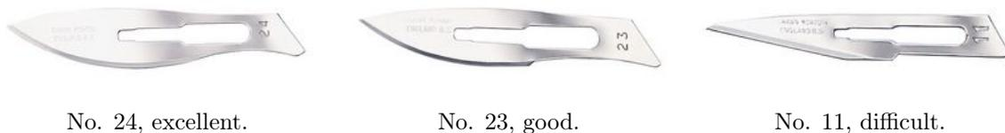
**Figure 3.2:** Scalpel blade shapes used (or tested) for ice cutting.
