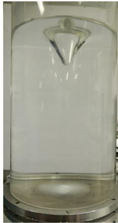
**Figure 3.10:** BFI vessel getting evacuated while being stirred with long stir bar, showing a small vortex on the surface.
