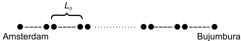
Figure 3.1: Quantum repeater. The division into segments is shown. The meeting point of two segments is called a repeater station or a node. The physical systems underlying different segments and nodes are identical.
