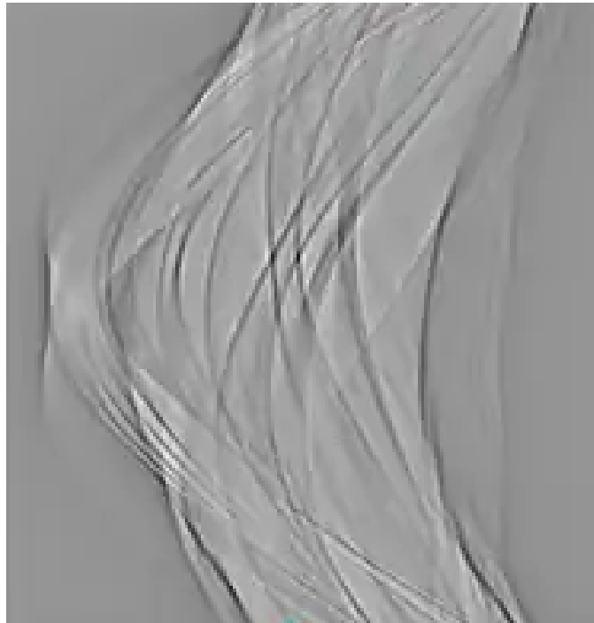
Figure 19: Sinogram in figure: 17, after application of the Ram-Lak filter. [10]
