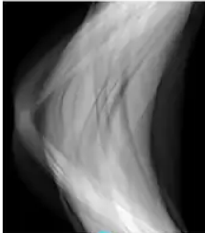
Figure 17: A sinogram made from a scan of figure: 16a. Horizontal lines in the sinogram is made from a single viewing angle. The vertical dimension is then created from many viewing angles. [10]
