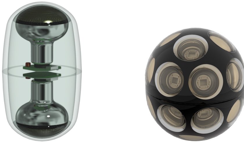
Figure 4.6: Two of the optical modules that are planned to be used for the IceCube Upgrade. Left: The D-Egg consists of two 8'' (20.32 cm) PMTs, one pointing upwards and one pointing downwards. Right: The mDOM consists of 24 PMTs of 3'' (7.62 cm), pointing almost isotropically in all directions.
