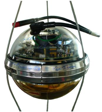
Figure 2.2: Original IceCube Digital Optical Module (DOM).
