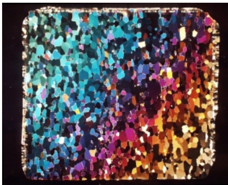
Figure 5.2: The sample from 2015.75 m depth. The change in dominant colour due to changes in thickness can be seen across the sample.
