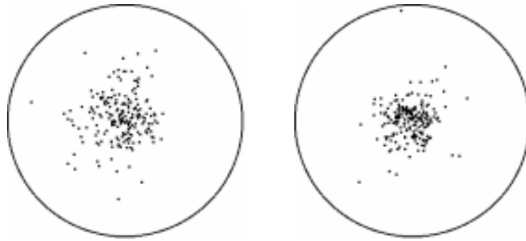
Figure 6.11: Fabric diagrams for the crystals inside a cloudy band (left) and outside (right) for the sample at 2029.18 m depth. 200 randomly chosen c-axes inside and outside the cloudy band respectively are plotted in the fabric diagrams.
