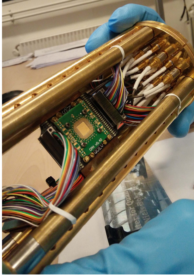
Figure 3.3: Puck with outer casing removed. A daughterboard, currently with no chip, is mounted in the center, with wires connecting it to the electrical lines of the cryostat.
