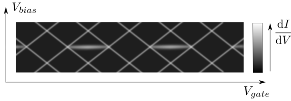
Figure 3.8: Diamond diagram showing the Kondo conductance at odd electron occupancy.
