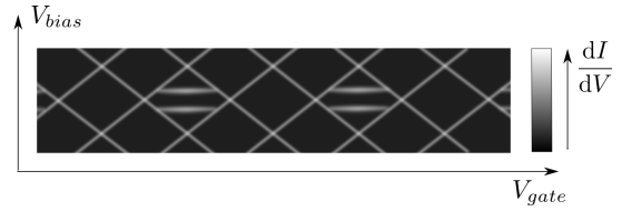
Figure 3.9: Split Kondo peaks due to the presence of a magnetic field B . For large bias voltages |V| \gg T_k the Kondo resonance will experience a cross-over to ordinary co-tunneling.
