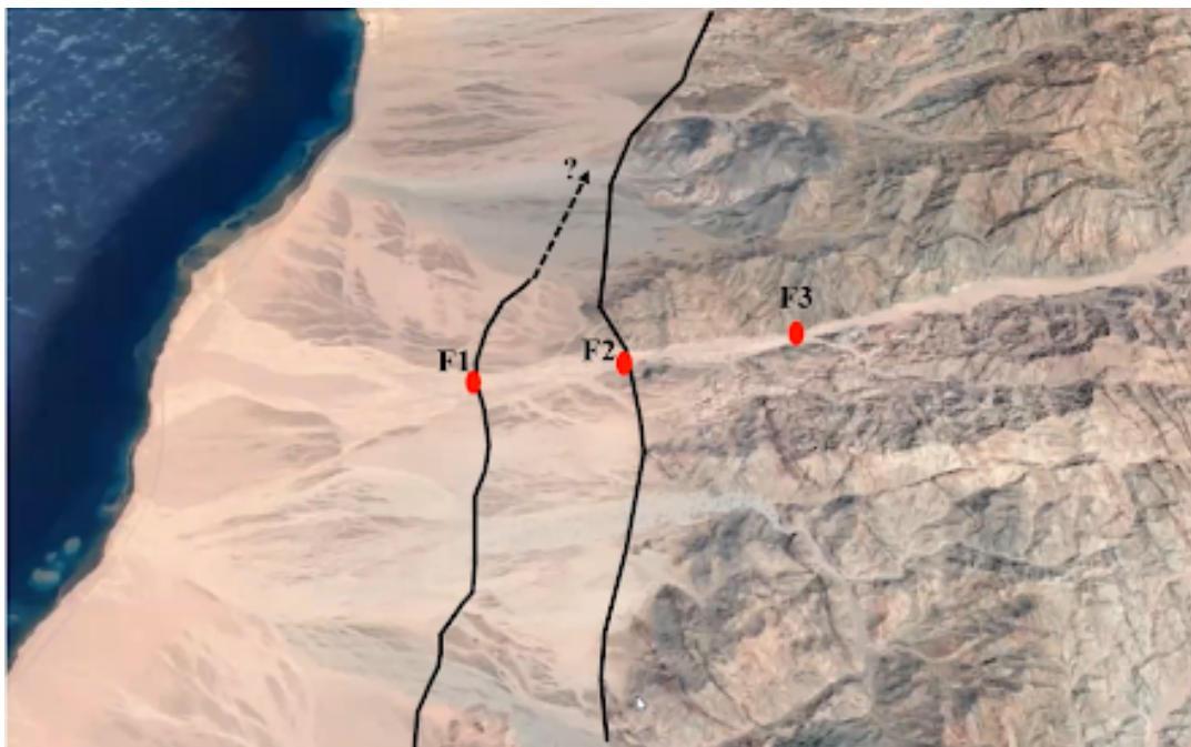
Figure 5.3.: Satellite image and confirmation of Faults F1 and F2, while F3 and F4 cannot be seen (Hanafy, 2022).
