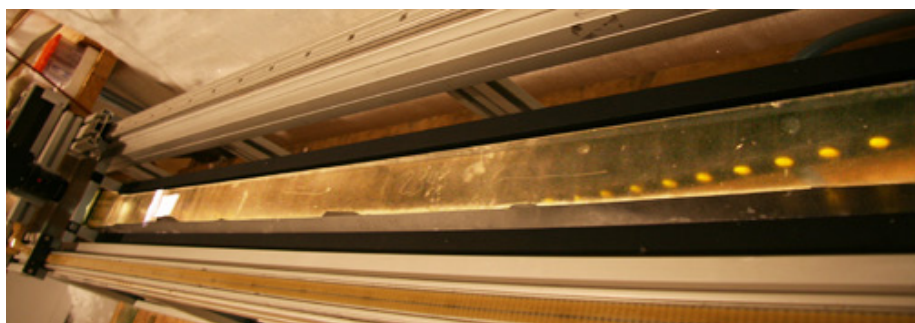
Figure 2.1: Picture of the line scan set up, with the camera in the left side. The top of a threebag was placed to the left. NEEM Field Dairy July 23 2009.
