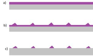
Figure 3: Different growth modes a) Frank-van der Merwe growth, layer-by-layer growth b) Stranski-Krastanov growth consisting of a wetting layer and island formation c) Volmer-Weber growth, only island formation
