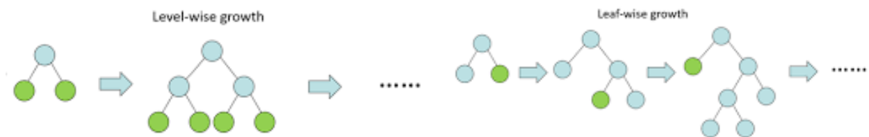
Figure 3.2: Graphical representation of the difference between level-wise and leaf-wise tree growth. Examples of algorithms using these methods of growing would be XGBoost using the level-wise tree growth and LightGBM using the leaf-wise tree growth.
