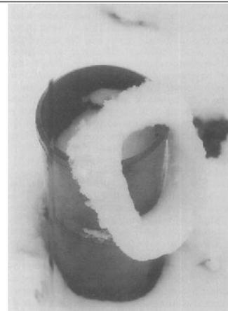
**Figure 2.5:** Rain gauge with clustered snow blocking the top.
