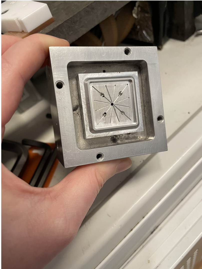
Figure 14: Photo of the melt-head with draining holes. Outer four holes are for fixation, only.
